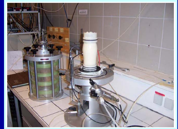
Bishop & Wesley triaxial cell and Fontainebleau soil specimen after test (TCD6, \sigma_c = 100 kPa)
